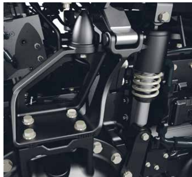
The suspended cab provides you a smoother ride whether on the road or in uneven terrain.
