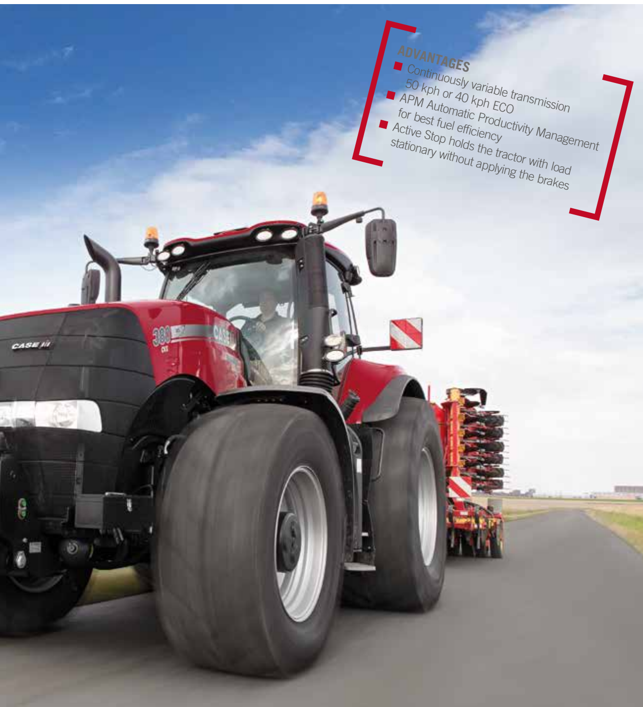
CVX transmission – stepless drive between 0-50 kph
