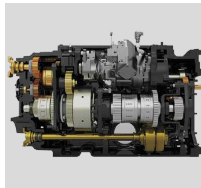
CVX transmission – stepless drive between 0-50 kph
